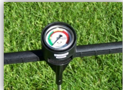
Figure 9. A soil penetrometer measures the pressure it takes to push the probe into the soil. It is a great tool to evaluate soil compaction.
