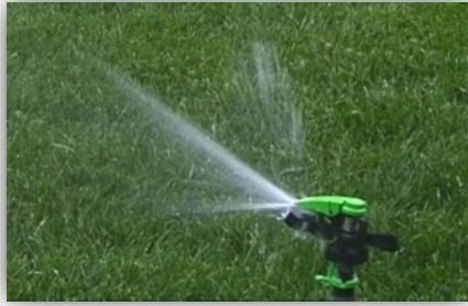
Figure 7. Impact or impulse heads rotate as the water stream coming from the nozzle hits a spring-loaded arm. Impact heads tend to experience fewer problems with marginal (dirty) water quality.
