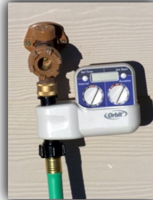
Figure 12. Single-zone controllers connect to the hose line. Left: This style is manually turned on and automatically turns off after a set number of minutes. Right: This battery powered controller turns water on and off at the day and time intervals set by the gardener.
