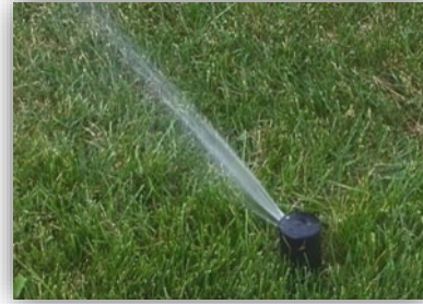
Figure 8. Gear-driven heads use the flowing water to turn a series of gears that rotate the head. Gear-driven heads are quieter to operate than impact heads.
