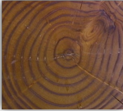
Figure 8. The “wood” of a tree is the xylem tissue. Xylem tissues that grew in the spring and early summer enlarge and are the tubes in which water with minerals flows from the roots to the leaves. In a cross-section of the log, these are light colored rings. Xylem tissues that grew mid-summer, at the end of the growth cycle, are higher in fiber content, creating a wall to the outside. In a cross-section of a log, these are the darker colored rings.
