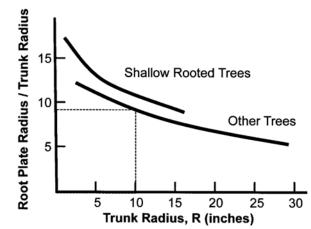
**Figure 14.** For example, a 10-inch trunk radius needs a root plate/trunk radius coefficient of 9. This would be 90" root plate radius (90"/10" = 9).
