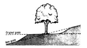
**Figure 6.** Using fills and cuts to improve PRZ for a tree on a slope.
