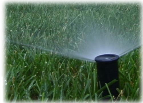
Figure 5. Pop-up spray heads are used for small areas, up to fifteen feet.
