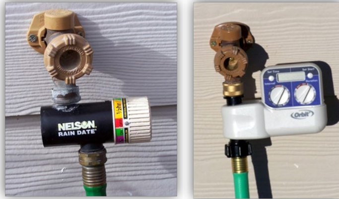
Figure 12. Single-zone controllers connect to the hose line. Left: This style is manually turned on and automatically turns off after a set number of minutes. Right: This battery powered controller turns water on and off at the day and time intervals set by the gardener.
