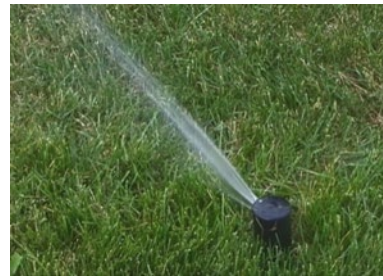
Figure 8. Gear-driven heads use the flowing water to turn a series of gears that rotate the head. Gear-driven heads are quieter to operate than impact heads.
