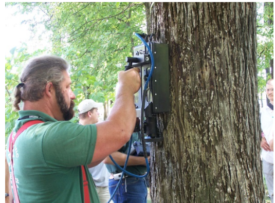
Figure 20 – Tree radar taking a look at the tree's internal wood structure.
