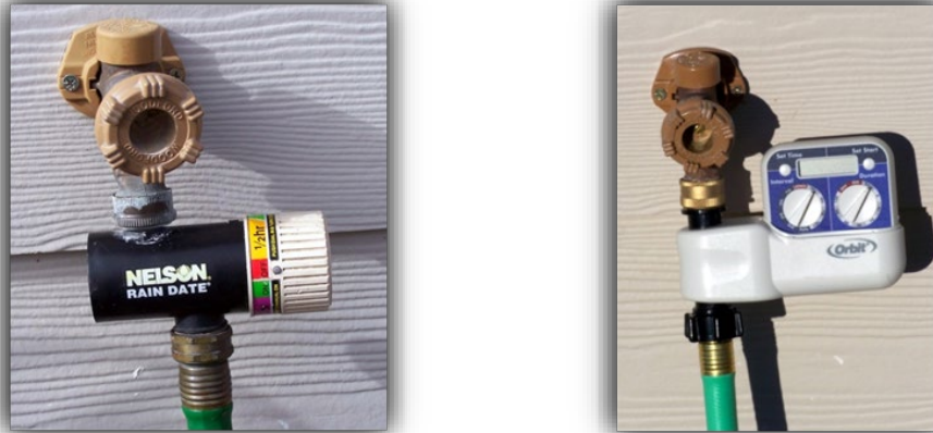
Figure 12. Single-zone controllers connect to the hose line. Left: This style is manually turned on and automatically turns off after a set number of minutes. Right: This battery powered controller turns water on and off at the day and time intervals set by the gardener.
