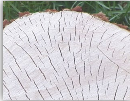
Figure 10. The cracks on this willow stump show ray cells.
